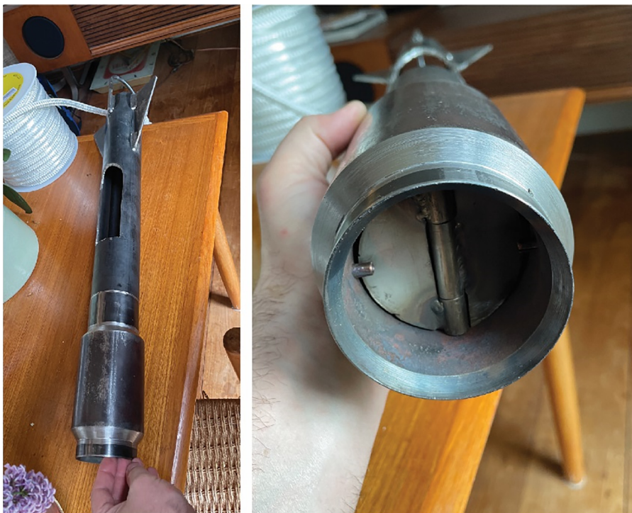
Fig. 4. Hornbrook sampler used to collect gytija at Regnault. See Bourdeau and Dyer (2023) for further details on this type of sampler.
